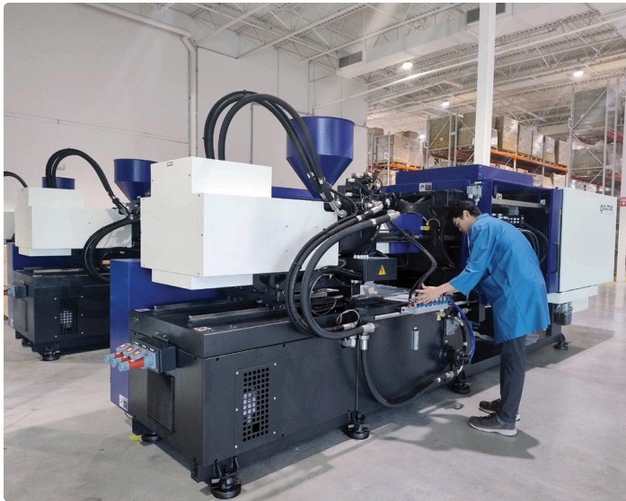
Injection moulding of device housings, Brossard plant.
