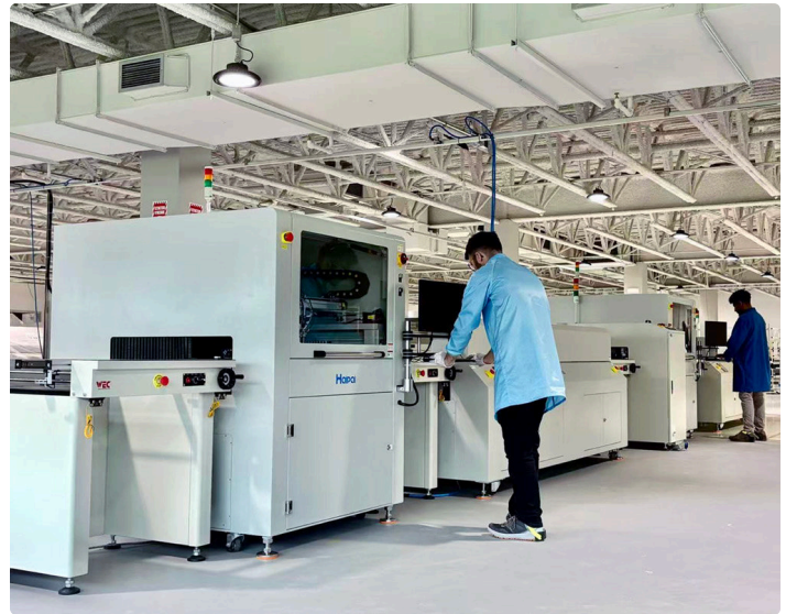
Surface-mount electronics assembly line, Brossard plant.
